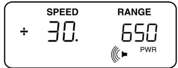
There is no need to clear the speed and range of a vehicle from the display before tracking the next vehicle.
