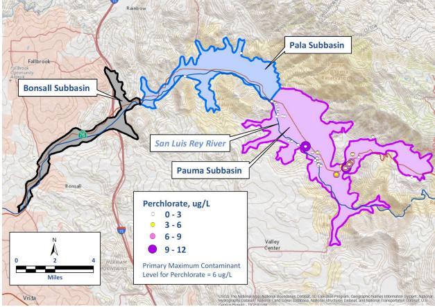
Figure 3-1. Historical Areas with Elevated Perchlorate Concentrations
