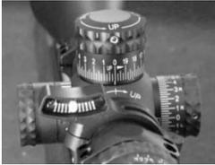
To “index” your turrets to 0,0: Loosen the set screws on the elevation and windage turrets and rotate the dial to 0. Tighten the set screws per your scope manufacturer’s instructions.
