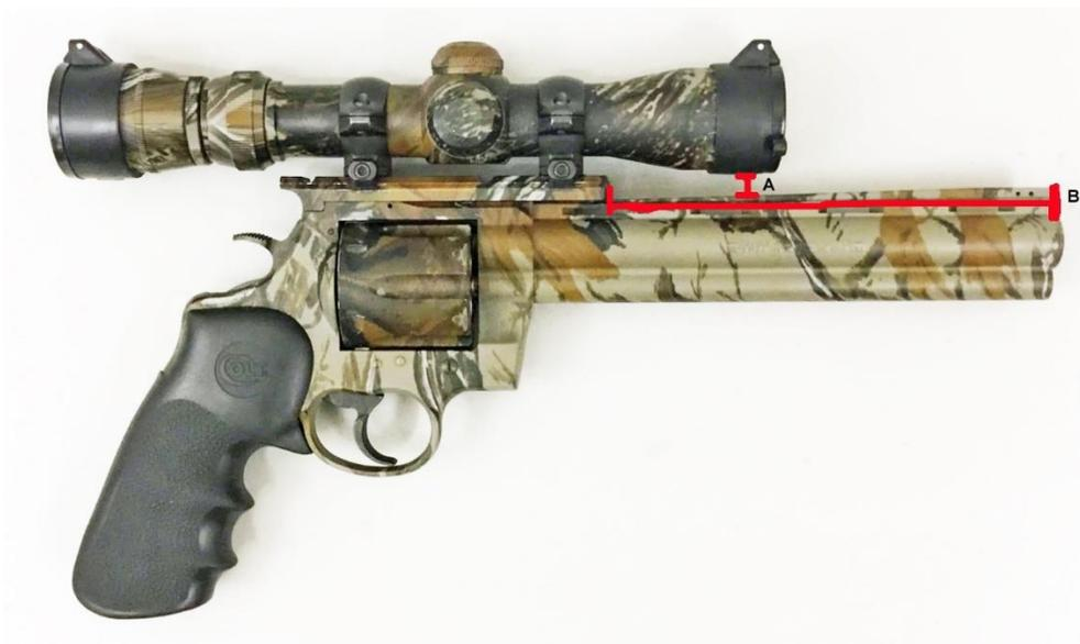
Criteria: The measurement from the end of the barrel to the optic or rail (B) must be 5 inches or more. The measurement between the barrel and the scope must be 3/8 inch or more (A). If your measurements meet the criteria, a custom holster can be built.
