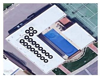
There is a solar heating system located on the pool building roof that consists of a Compool LX-22 controller and 20 solar panels that acircular coiled black tubing. This system was installed by General Solar and they previously advised that this system should last 20 years. The cost to replace the solar tubing in 2016 was about \$400 per unit, and the cost to replace the controller was \$700. We have adjusted these costs for inflation.
