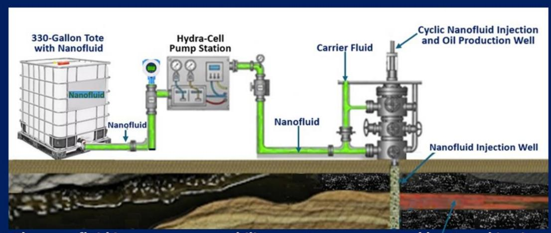
The nanofluid increases permeability, creates pressure and heat, and in-situ surfactant alters wettability and reduces interfacial tension.
