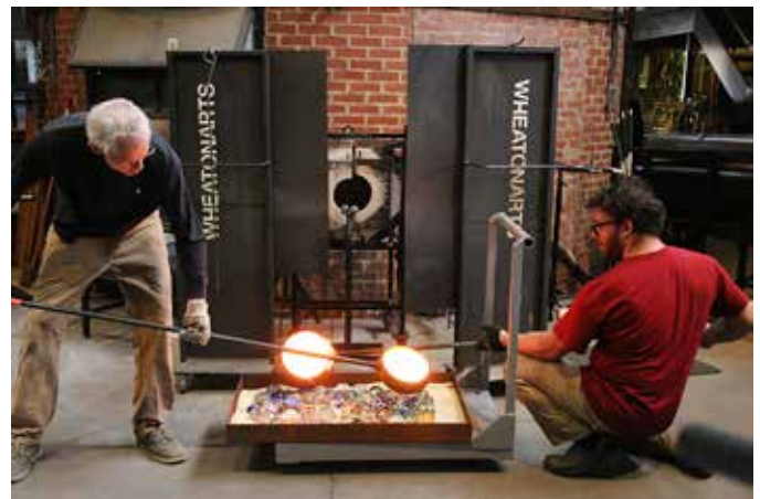
WheatonArts workers pouring hot glass over defective parsley weights
