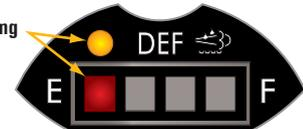
Vehicle speed limited to 5 mph / engine derated
