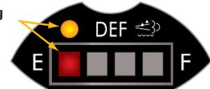
Vehicle speed limited to 55 mph / engine derated
