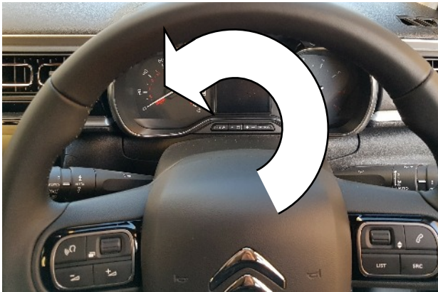
CHECK AROUND YOU. THEN SLOWLY START TO MOVE BACKWARDS & STEER QUICKLY LEFT FULL LOCK
