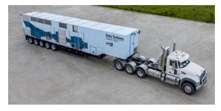
The Solar Turbines SMT 130 is a mobile gas turbine designed for power generation and mechanical drive applications. It is known for its compact design, high efficiency, and reliability. The SMT 130 typically operates on natural gas or other gaseous fuels and is suitable for various applications, including oil and gas, industrial processes, and power plants.
