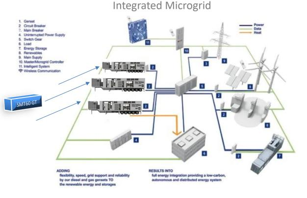
"The Solar Turbines' SMT 60 and SMT130 gas turbine can serve as the anchor of many microgrids. If the plant has the ability to island, which essentially makes it a microgrid, the gas turbine is a critical part. It is key to load control, frequency control and voltage control. It is the heart behind the microgrid." 1
