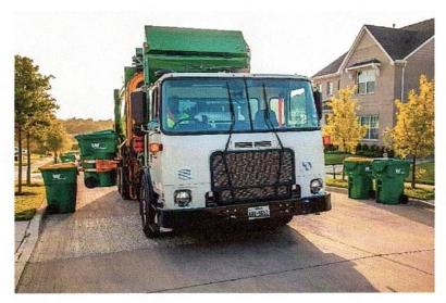
Operated by a single driver from inside the truck, the automatic side loader utilizes a mechanical arm with a claw to pick up a cart from the curb. When grasping onto the cart, the claw makes a secure grip around the widest part of the cart body. After gripping onto the cart, the mechanical arm lifts the cart up, dumping waste into the top front of the garbage truck.
