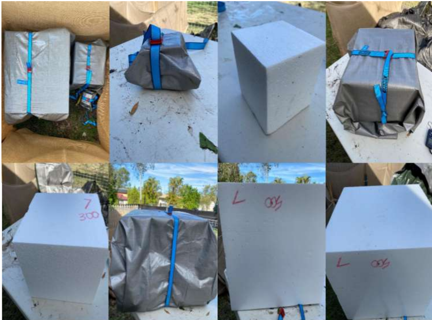
Supp Fig 7. Treatment 7: heavy duty tarp at the beginning of experiment (A); the 0.1 m 3 piece at the end (B-C); the 0.3 m 3 piece at the end (D-E); and the 0.5 m 3 piece at the end (F-H).
