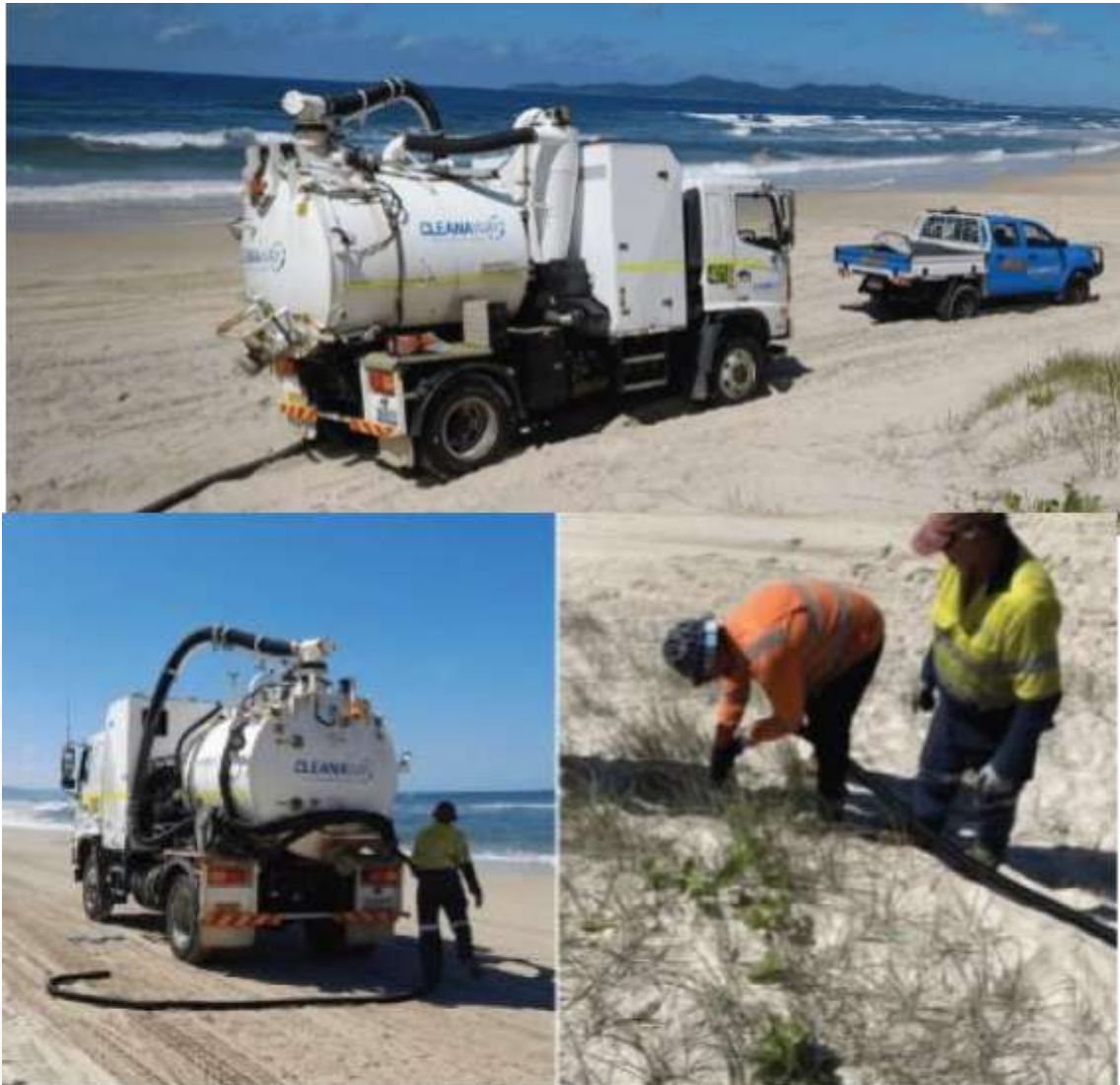
Figure 16. CleanAway Queensland all terrain truck removing polystyrene from the beach (Image credit: Sharyn Kerrigan).
