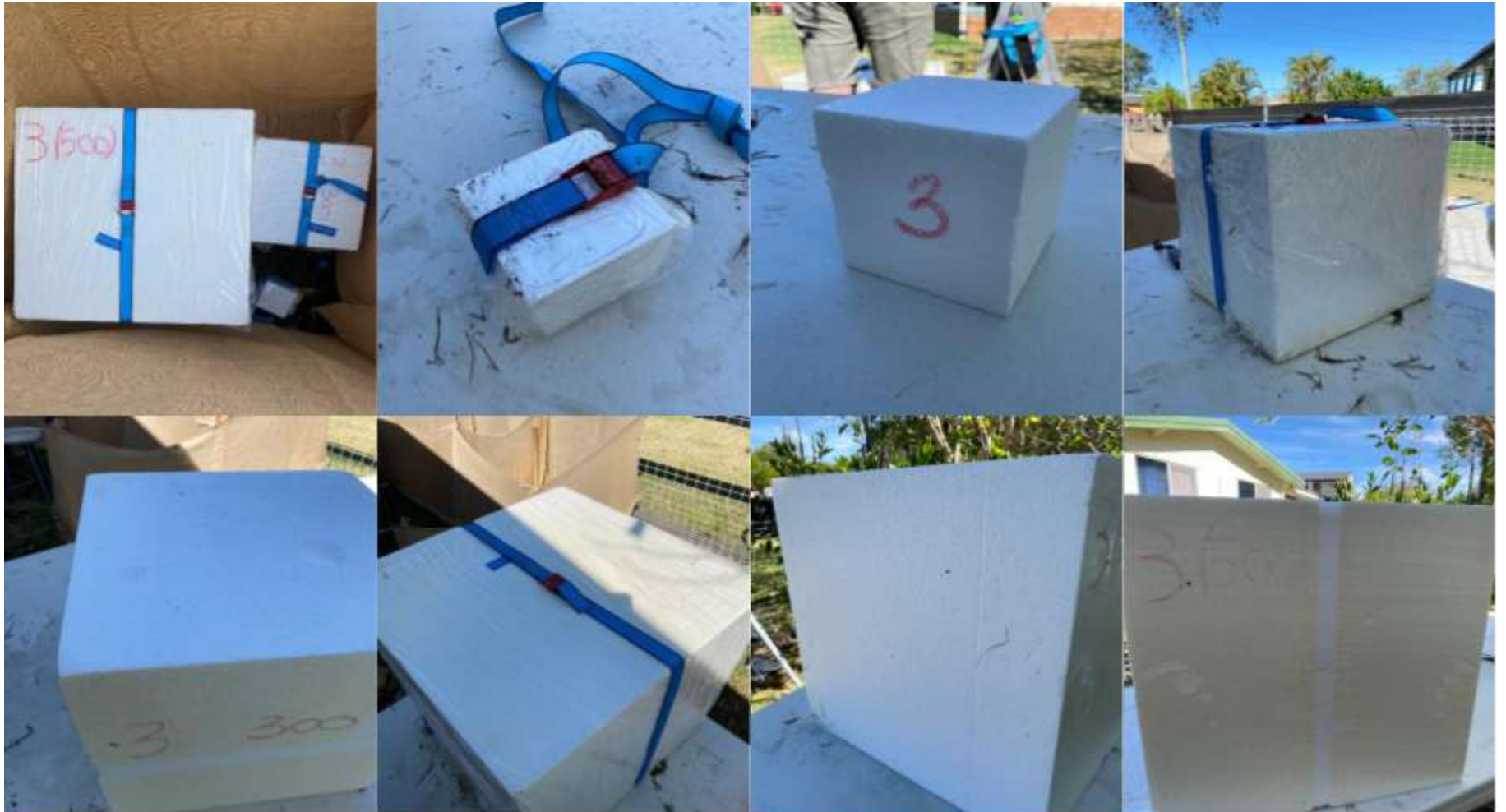
Supp Fig 3. Treatment 3: heavy shrink wrap (25 \mu\text{m} thickness) at the beginning of experiment (A); the 0.1 \text{m}^3 piece at the end (B-C); the 0.3 \text{m}^3 piece at the end (D-E); and the 0.5 \text{m}^3 piece at the end (F-H).
