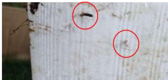
Figure 20 Control treatment with items growing out of the polystyrene (indicated in the red circles).
