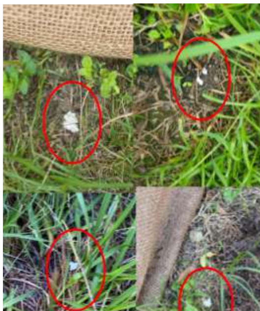
Figure 21. Polystyrene leakage in the primary barrier from the control treatment (top) and the biodegradable hand stretch wrap (bottom).
