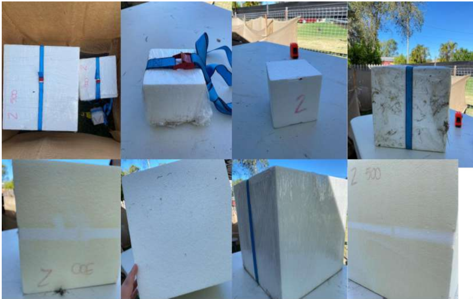
Supp Fig 2. Treatment 2: light stretch clear shrink wrap (17 \mu\text{m} thickness) at the beginning of experiment (A); the 0.1 \text{m}^3 piece at the end (B-C); the 0.3 \text{m}^3 piece at the end (D-F); and the 0.5 \text{m}^3 piece at the end (G-H).
