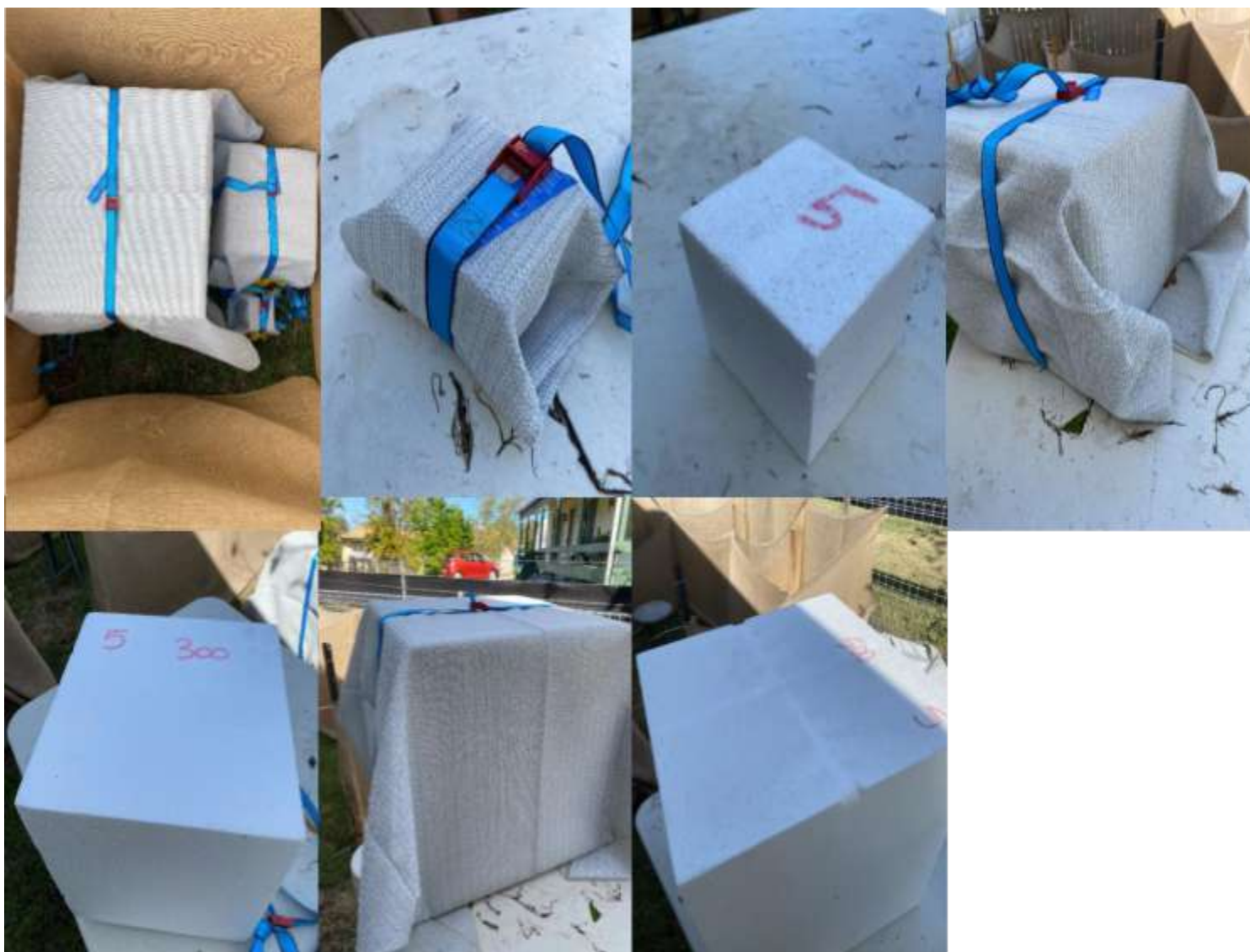
Supp Fig 5. Treatment 5: shade cloth silver (90% UV heavy duty cloth) at the beginning of experiment (A); the 0.1 m 3 piece at the end (B-C); the 0.3 m 3 piece at the end (D-E); and the 0.5 m 3 piece at the end (F-G).
