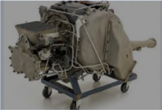
Typical version of the front drive Turbine Notice the transmission tail protruding
