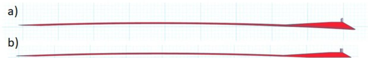
**Figure 13.** Comparison of control wing section (a) to wing section with trailing section of lower concave surface replaces with horizontally-flat surface(b).
