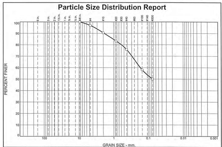
% Gravel % Sand % Fines % +3" Coarse Fine Silt Fine Coarse Medium Clay 0.0 0.0 3.0 6.5 14.6 25.8 50.1
