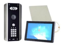
Keypad includes 3 relays, 1200 codes, with latching & momentary operation & more. Modern blue back lighting effect.
