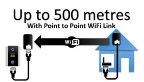
Range can be extended up to 500 metres by using various open market devices, such as
