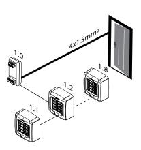
An ESPAS30 installation can be implemented with the management of pedestrian entry points, using the Axxedo system.
