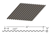
The PBD panel is an exposed-fastened panel system that can be used for roof and wall applications. When used in wall applications, panels can be installed vertically or horizontally. The ribs in the PBD panel are symmetrical from top to bottom, which makes this panel ideal as a roof liner.
