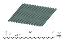
The PBC panels can be used for both roof and wall applications. PBC panels are attached to a building structure with exposed fasteners and is often used in horizontal applications on walls.
