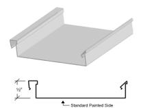
QwikLok™ panels are ideal for underhung applications; no more fighting with trying to install two panels at one time. Unlike conventional roofing cover, QwikLok™ panels can be assembled from the underside of the structure one panel at a time, producing a flush appearance with no exposed fasteners. The standard QwikLok™ panel is painted on the bottom side. Please specify if the panel should be painted on the top side.
