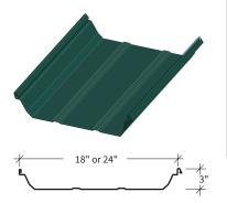
The Ultra-Dek® roof panel is a snap-together, trapezoidal leg standing seam roof system. Ultra-Dek® panels are available in 18-inch and 24-inch widths. Ultra-Dek® requires a minimum slope of 1/4:12 and is ideal for industrial, commercial and architectural applications. Ultra-Dek® can be erected on various types of construction.
