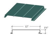
The FW-120 panel is a concealed-fastened wall and liner panel that provides a flat appearance. FW-120 is commonly used for architectural, commercial and industrial markets. The heavy gauge offering provides for large spanning capabilities, particularly in composite wall applications.
