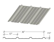
The PBR panel is commonly used for a wide variety of architectural, agricultural, commercial and industrial applications. PBR is a structural, exposed-fastened panel that can be used for both roof and wall applications. The minimum roof slope for PBR is ½:12.
