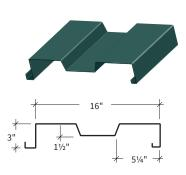
ShadowRib™ is a three-inch deep panel that combines aesthetics, economy and function to bring definition to metal structures. ShadowRib™ is a proven performer and a versatile tool to the designer. Structural strength in the ShadowRib™ panel is accomplished without sacrificing appearance or design flexibility. The fluted face creates distinctive shadow lines.
