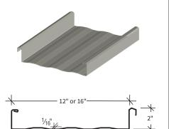
SuperLok® is a mechanically field-seamed system that combines a 2" tall slim rib with exceptional uplift resistance. MBCI designed the SuperLok® system to withstand the most rigorous weather conditions. This panel can be installed directly over purlins or bar joists, and does not require a solid substructure for support.
