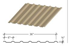
The PBU panel is an exposed fastener system that can be used for both roof and wall applications and can be installed directly over purlins or joists. PBU offers the versatility of being used in both vertical and horizontal applications to give designers a contemporary appearance for their building project. PBU is recommended for 1:12 or greater roof slopes.
