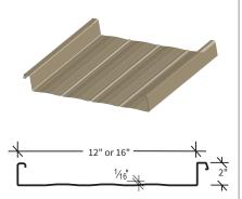
BattenLok® HS is a mechanically field-seamed, high strength structural standing seam roof system. The BattenLok® HS panels have a two-inch tall vertical seam and are available in both 12-inch and 16-inch widths. BattenLok® HS can be installed directly over purlins or bar joists and is capable of transitioning from roof to fascia. BattenLok® HS does not require a solid substructure for support.
