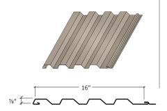
MasterLine 16 is a concealed-fastener metal wall panel that provides an interesting shadow line, enhancing the aesthetics of the panel. While primarily designed for horizontal applications, it can also be installed vertically to give a distinguished architectural design. The panels provide 16-inch coverage and are available with factory-applied mastic in the side laps. Panels may be attached to metal studs, with or without sheathing, as well as to subgirts.
