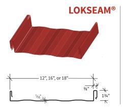
LokSeam® is a snap-together standing seam roof system with a 1¾" tall vertical rib for use on roofs with a minimum slope of 3:12. Available in 12-inch, 16-inch and 18-inch widths, LokSeam® panels can be installed over open framing or a solid substructure and are capable of transitioning from roof to fascia with the use of a rib cover. LokSeam® does not require a solid substructure for support.
