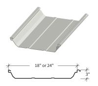
The Double-Lok® roof panel is a mechanically field-seamed, trapezoidal leg standing seam roof system. Double-Lok® panels are available in 18-inch and 24-inch widths and require a minimum slope of ¼:12. Double-Lok® panels are ideal for industrial, commercial and architectural applications.
