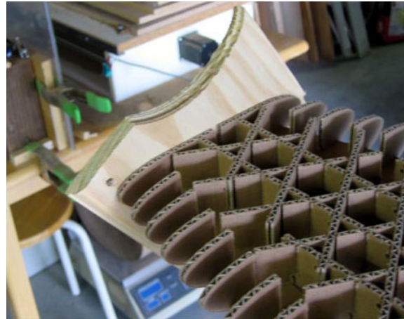
Mike Sheldrake 2008 - isogrid surfboard - cardboard, fiberglass & epoxy resin
