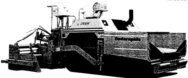
Crawler rubber track paver with a turbocharged Cummins 4BTA 3.9L in-line 4 cylinder diesel engine, 8' (2438 mm) screed, hydraulic vibration, one-piece pull arms, 14" (355 mm) diameter
