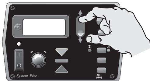
Figure 5-3. Center the Tow Point Cylinders
