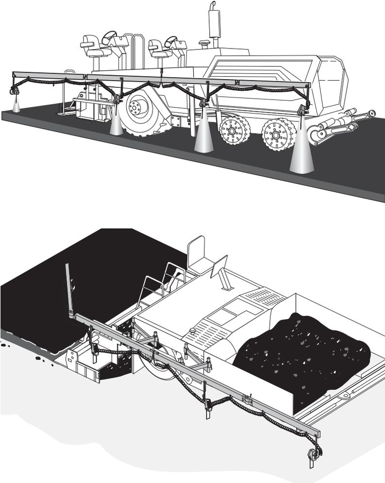
Figure 6-22. Example Placement of SAS Trackers Over Reference
