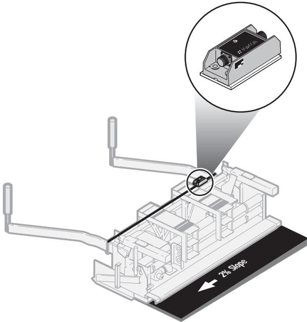
Figure 2-29. Position of Slope Control on Paving System
