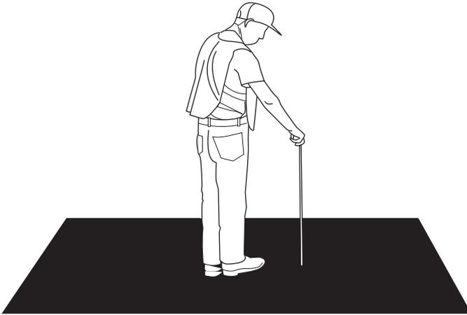
**Figure 5-9. Checking Pad Thickness**
