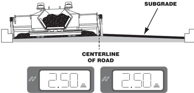
**Figure 7-9. Second Pass when Paving Uneven Curbs**
