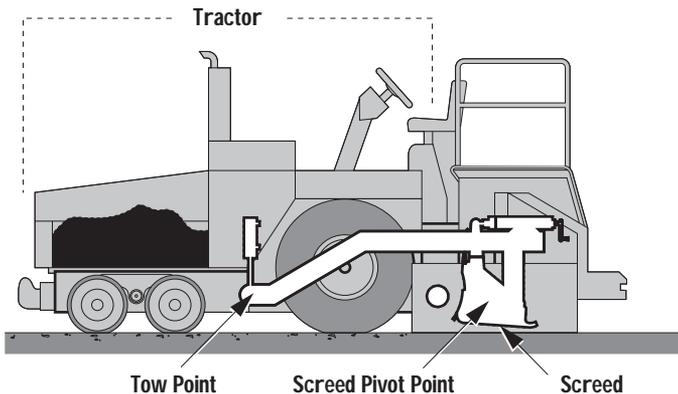
Figure 2-1. Paver Components
