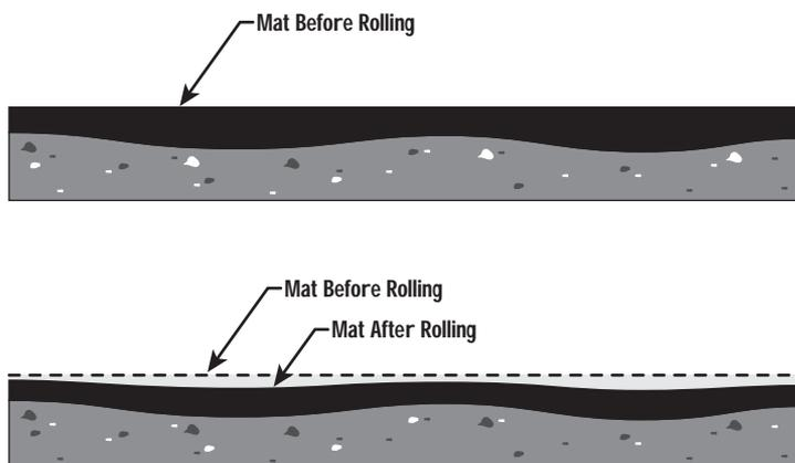
Figure 2-15. Differential Compaction
