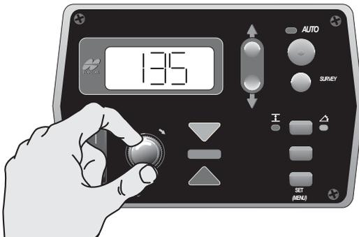
Figure 4-30. Setting the Raise Valve Offset Value
