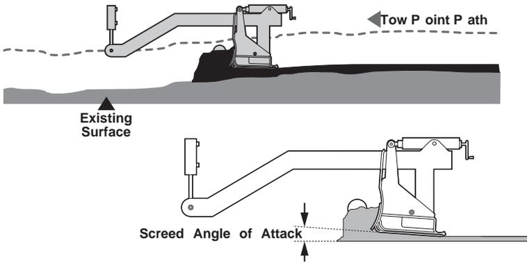
Figure 2-2. Tow Point Path and Planing Angle
