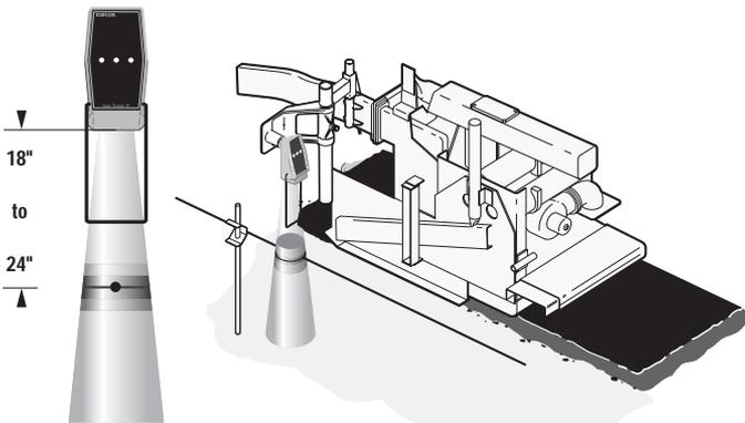
Figure 6-8. Tracker Position – Mat laid at Specific Elevation.
