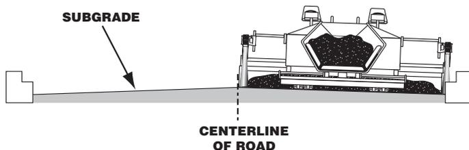
Figure 7-2. Positioning Tracker Over Gutter
