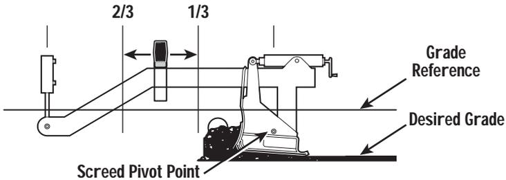
**Figure 6-10. Correct Tracker Placement in Relation to Scream**
