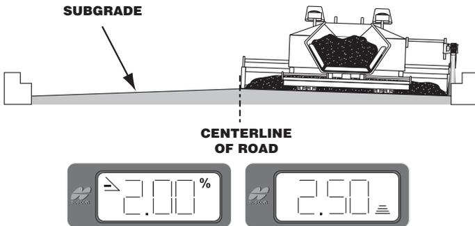
**Figure 7-8. Paving Uneven Curbs with Slope Control**
