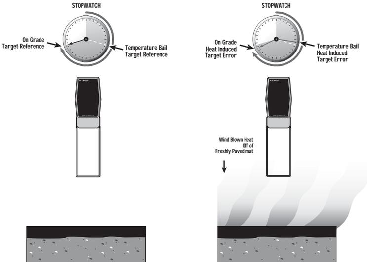
Figure 2-24. Working with Sonic Trackers and Temperature Changes
