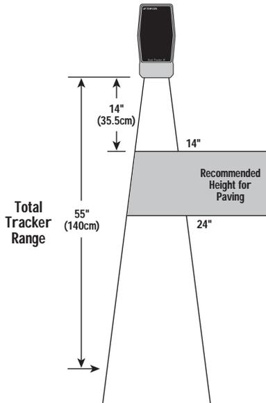
Figure 6-1. Recommended Tracker Placement
