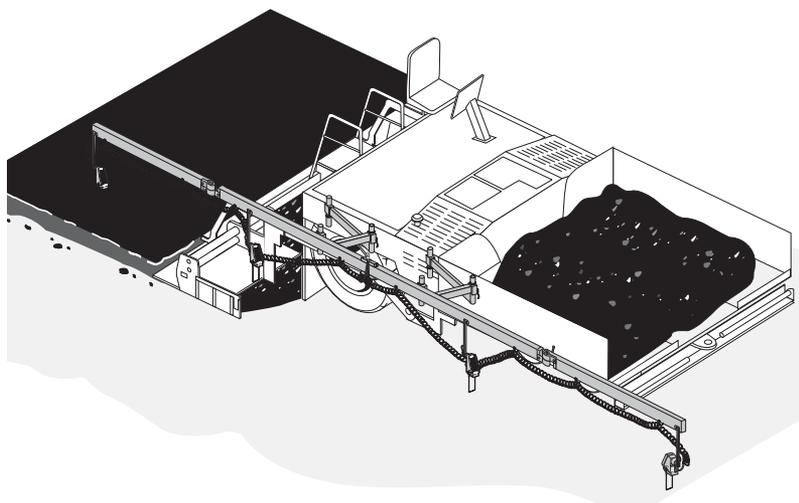
**Figure 6-23. SAS Setup when Screed Extension is Unsatisfactory**
