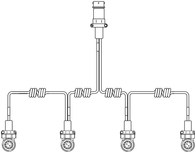
**Figure 6-20. SAS Cable Connectors to Sonic Trackers**
