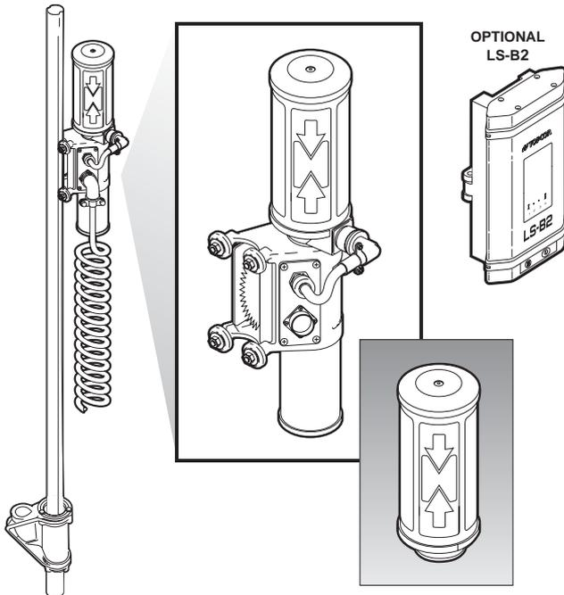
Figure 1-7. Laser Tracker & Trackerjack
