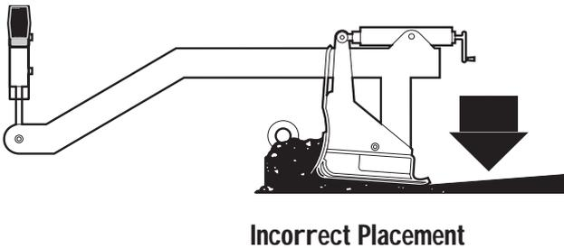
**Figure 6-14. Tracker at Tow Point Causes Erroneous Corrections**
