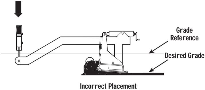
**Figure 6-13. Incorrect Placement of Tracker at Tow Point**
