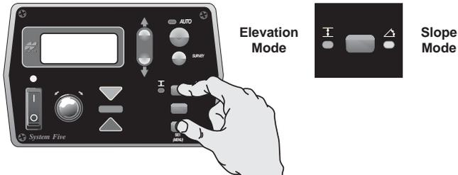
Figure 4-15. Slope/Elevation Button
