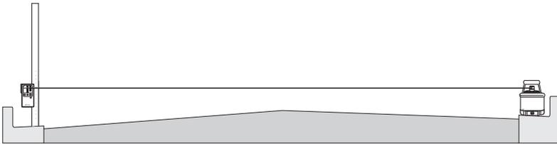
**Figure 7-10. Checking Curb Elevations**
