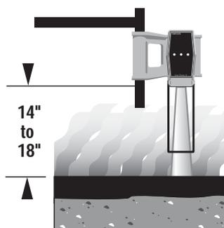
Figure 6-6. Temperature Conditions and Tracker Placement
