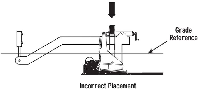
**Figure 6-11. Incorrect Placement at Scream Pivot Point**
