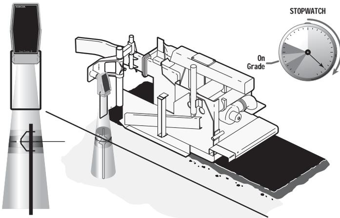
**Figure 2-23. Obstructions within the Sonic Tracker's Working Window**
