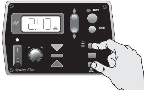
**Figure 7-18. Switching to Elevation Control and Surveying On-grade**
