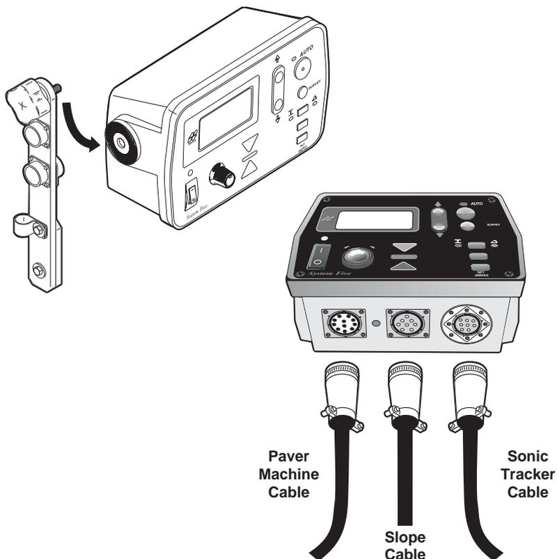
Figure 5-1. Attach Control Box and Connect Cables
