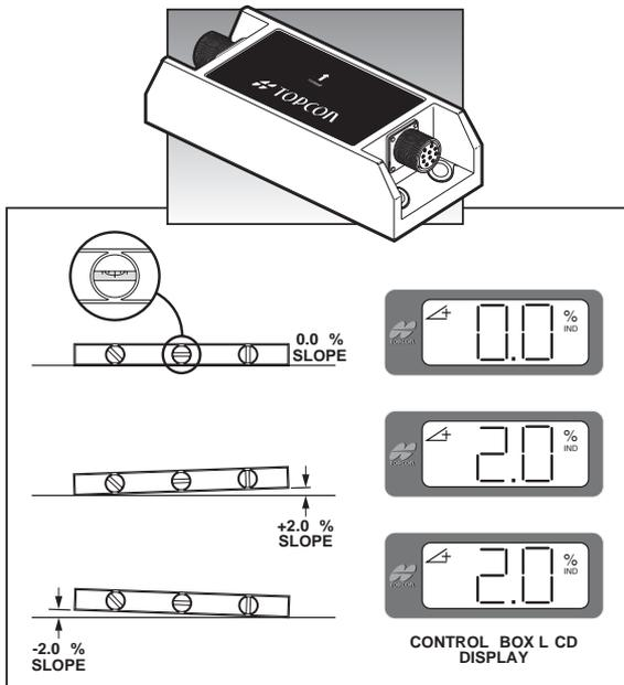
Figure 1-5. Slope Sensor
