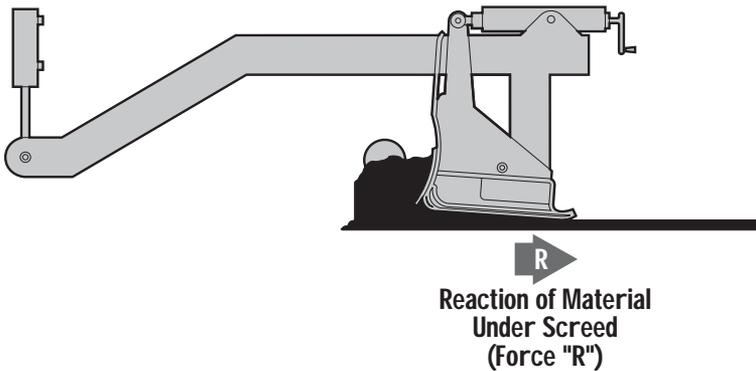
Figure 2-12. Reaction of Material Under Screed
