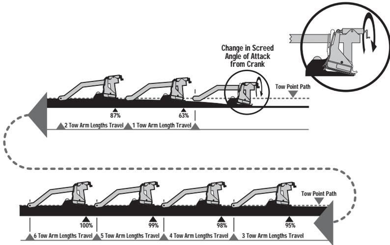
**Figure 2-5. Manually Changing Mat Thickness**
