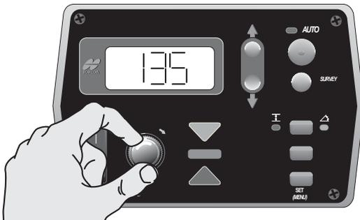
**Figure 4-32. Setting the Lower Valve Offset Value**
