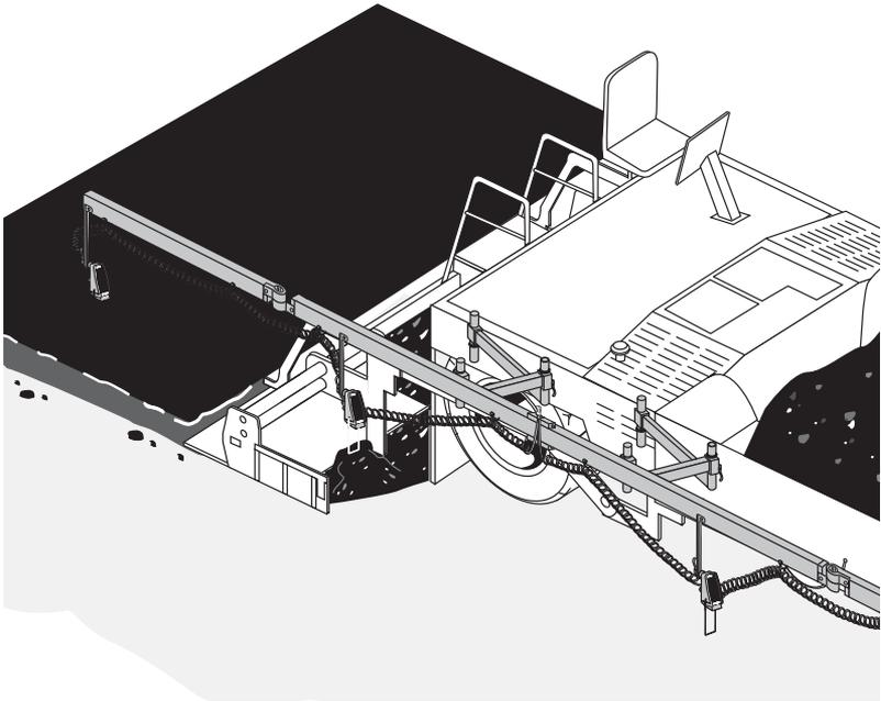
Figure 6-24. Repositioning the Sonic Tracker
