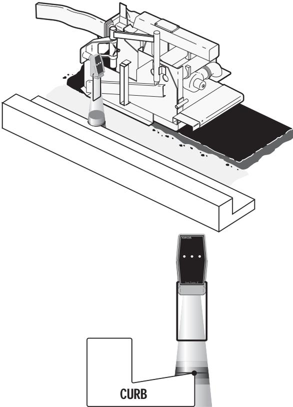
Figure 6-3. Position of L-Bar with Tracker on Bracket
