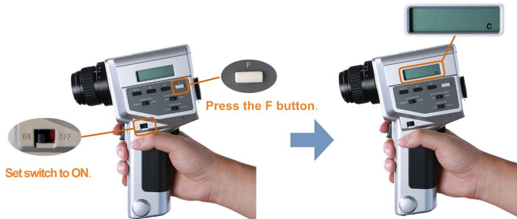
Figure 12-7 Setting CS-100A colorimeter
