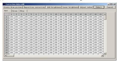
① Correction by hand: Select the color that needs to be corrected (red, green, blue), and choose the pixels that require to be corrected, using ctrl key can select
