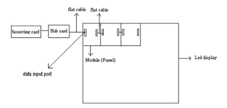
5. Data type, (red, green, blue) red, green and blue unite as one, three colors serial; red, green and blue unite as one, four colors serial. Generally speaking, the first data type (Red, green, (blue) separately) for Led display, the other items for light-decoration.
