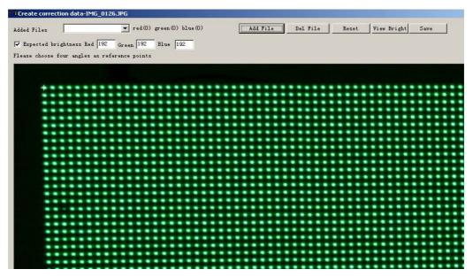
When select the picture, make sure every pixel is inside the four corners. After selecting, computer will mark all the pixels, as shown in below figure.
