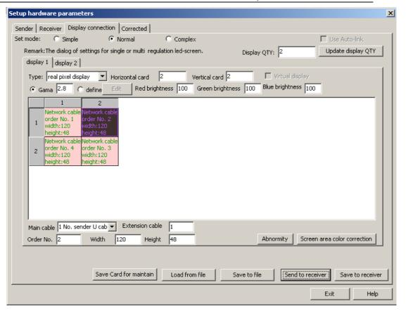
The upper box means: one sending card supports two displays, one (Display 1) uses the U port of the sending card, the other (Display 2) using the D port of the sending card.
