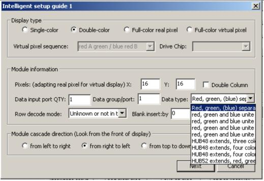
6. Choose the row decode mode (Unknown or not in the following options\static, no decode\no decode chip, row drive directly, with OE\no decode chip, row drive directly, no OE\chip 138 decode\chip 139 decode\chip 145 decode\chip 145 decode\chip 154 decode\chip 164 decode\chip 192 decode\chip 193 decode\chip 595 decode\chip 4094 decode)
