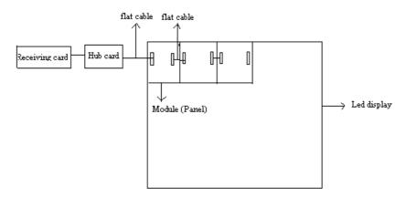
4. Input the quantity of the data input port, and the quantity of data group for every data input port, taking the full-color as an example, data input port-- how many data input ports at back of each full color module; Data group-- how many R, G, B data groups for a full color module. as shown in below figure
