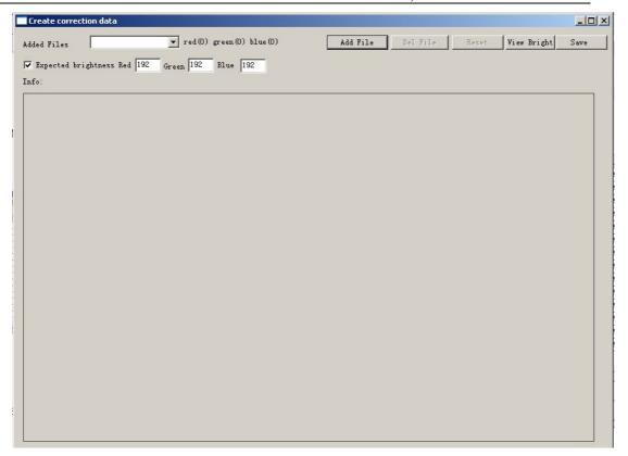
And click "Add file" to add the pictures; then click the four corners of the LED display in the picture or parts of the led display that user wants to balance the brightness.
