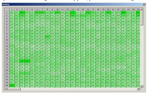
Select all the pictures of the led display/cabinet, the software will recognize how many pictures for each color (red, green, blue), and mark the value of lowest brightness pixel, highest brightness pixel and most pixels with same brightness. As shown in below figure.
