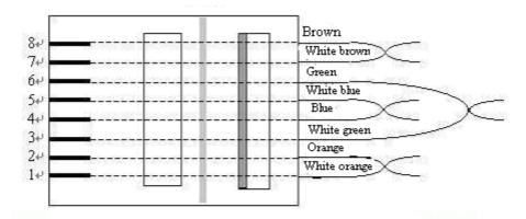
RJ45 Connector TIA/EIA 568B Criterion
