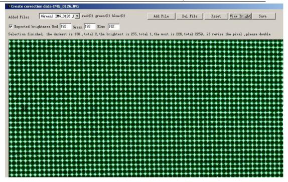
Check all the marked pixels, if error, click "Reset" for reselecting the four angles/corners for the picture;
