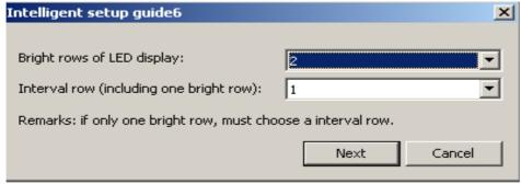
Notice: Interval rows mean how many black (dim) rows between two bright rows, and then add one bright row for the total interval rows. (You must figure out all the bright rows in the panel, but for the interval rows, you only need to figure out how many rows between two bright rows.) For example, as shown in below figure, there is one black (mid) row between two bright rows, choose 2 (1+1=2) rows for the interval rows, 4 rows for bright row.
