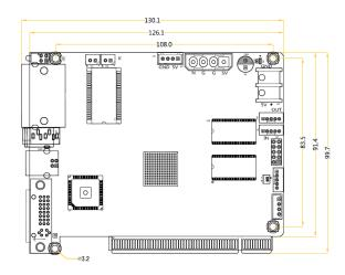
Tolerance: ±0.3 Unit: mm
