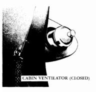
To stop the flow of air, push the ventilator tube all the way in.
