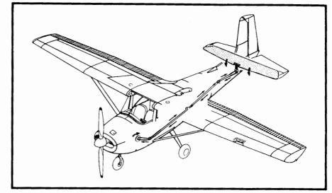
Figure 27. Adjustable Stabilizer Control System
