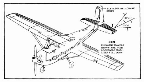
Figure 26. Elevator Control System
