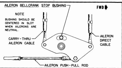
Figure 24. Aileron Bellcrank Adjustment
