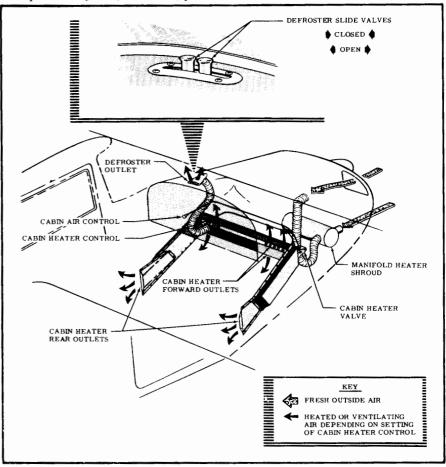
Figure 9. Cabin Air Temperature System
