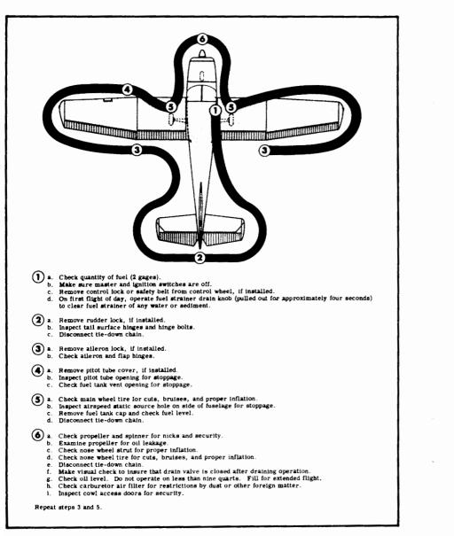
Figure 10. Exterior Inspection Diagram
