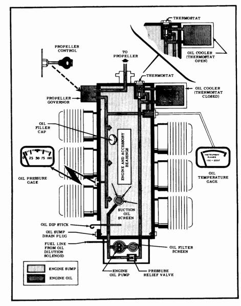
Figure 3. Oil System Schematic
