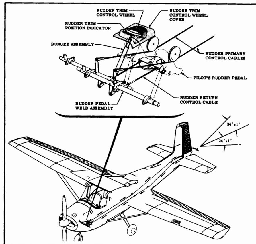
Figure 25. Rudder Control System
