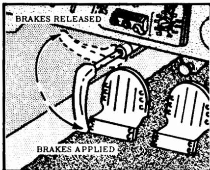
**Figure 8. Parking Brake Operation**
