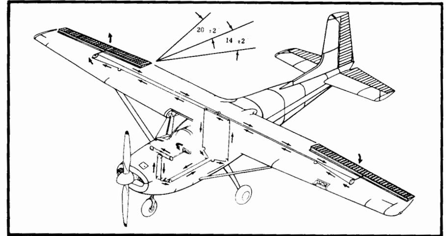
Figure 23. Aileron Control System
