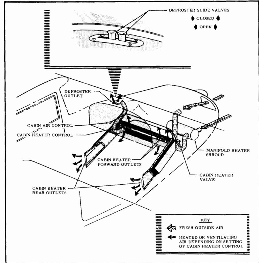
Figure 9. Cabin Air Temperature System
