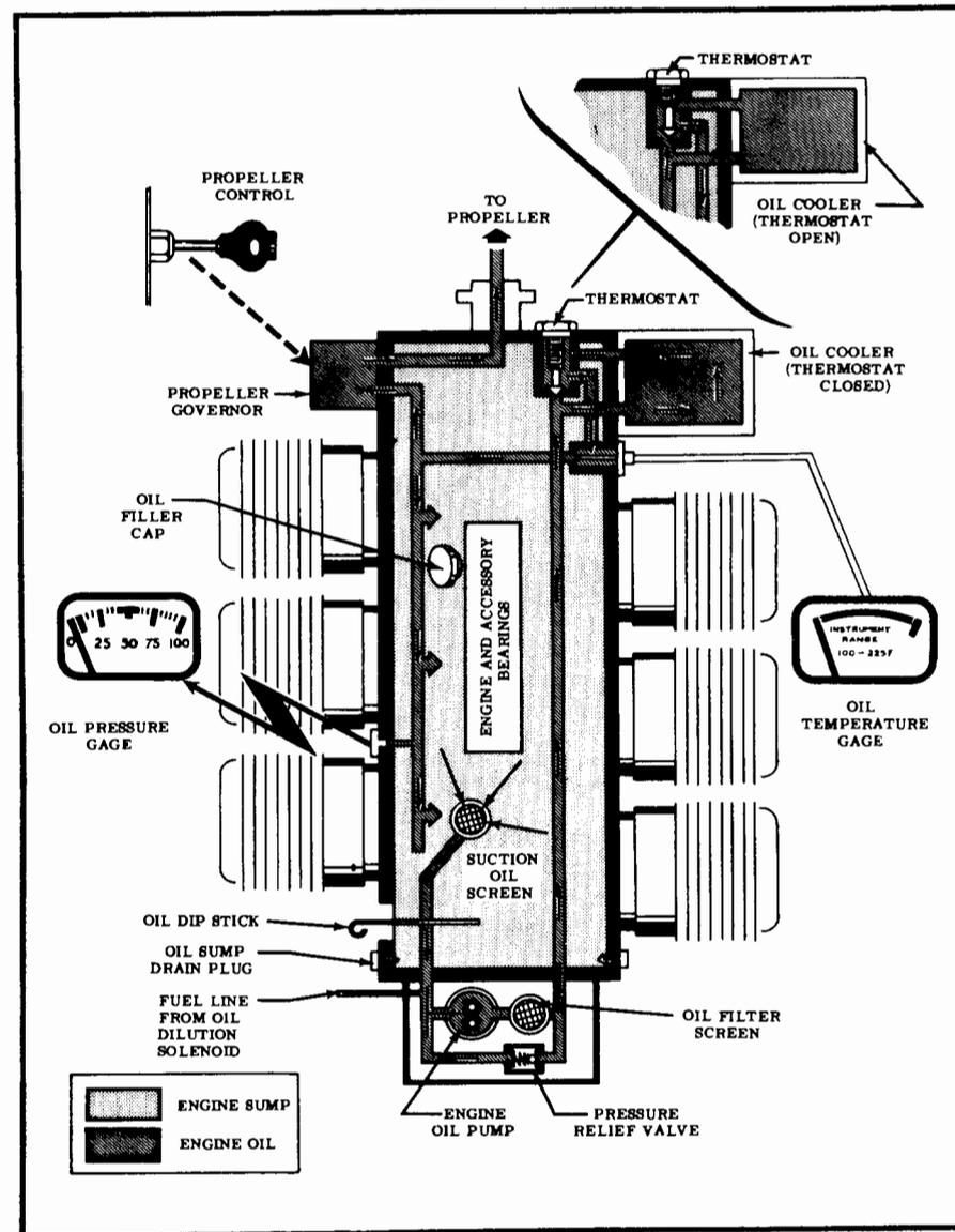
Figure 3. Oil System Schematic
