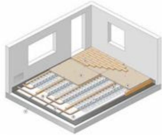
Radiant In-Floor Heating
