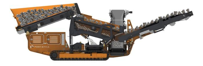
However with 5 seconds and without the need to de-assemble any part of the machine, the oversize conveyor can be retracted so that this conveyor captures both the midsize and oversize product. The combined product is then stockpiled out the front oversize conveyor.
