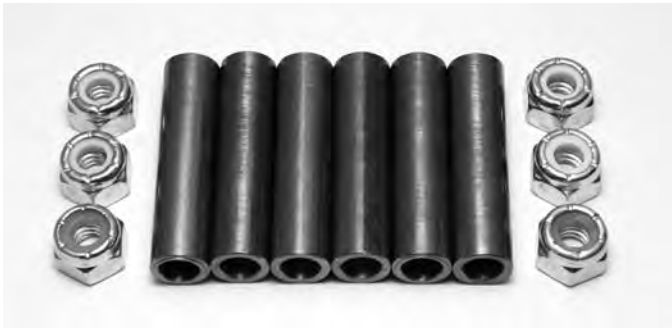
Clutch Backing Plate Stud Spacer Kit OEM style spacers and locknuts used on 1979-Early 1984 Sportster. Available in standard length and undersized. Stock No. 2756-12 Standard Stock No. 2765-12 -.040 Undersized Stock No. 2775-12 -.080 Undersized
