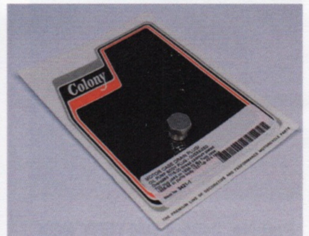
Part No. 3421-1 MOTOR CASE DRAIN PLUG/OIL PUMP BODY PLUG - OVERSIZED Oversized 7/16-20 thread cadmium plated 700 plug used on 1936-70 Big Twin case, 1968-84 oil pump body, 1937-up 45's case Retail: $3.30
