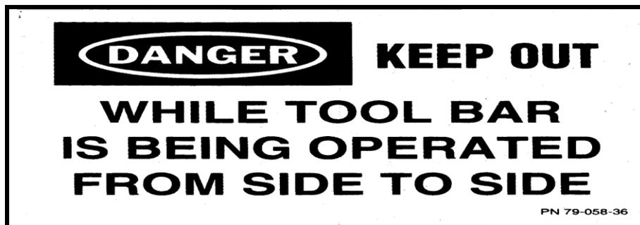
Tool Bar Guide Decal: Located on Right and Left Front Side of Tool Bar Guide
