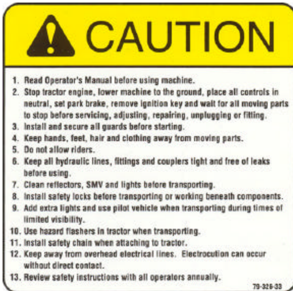
P/N 79-326-33 Location: Vertical tongue frame, below rake control valve.
