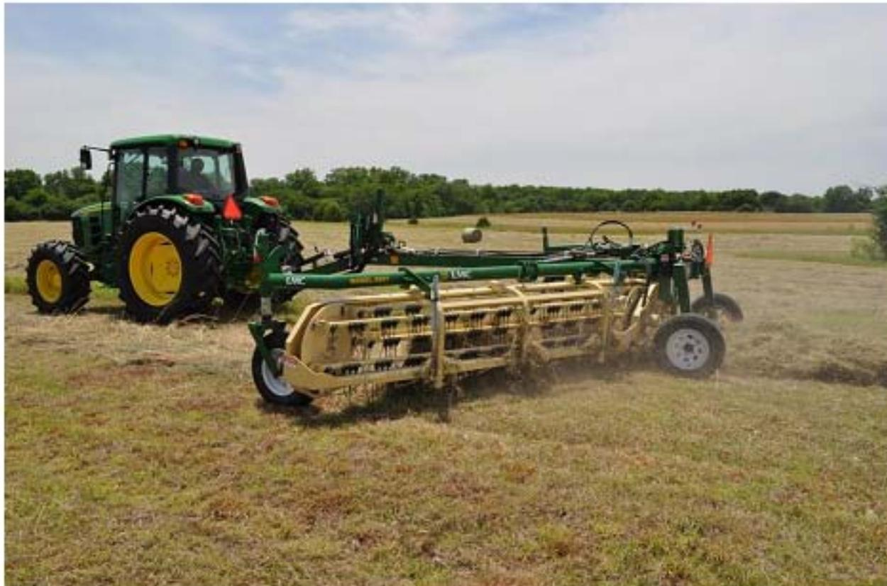
Hydraulic Cylinder (once folded, this raises the front of the rake for transport position. Note: There is a cylinder lock on the cylinder that needs to be removed.)
