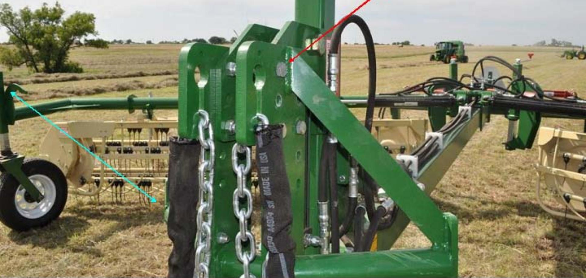
Make sure that these adjustments are made with the cylinder down. Once the rake is folded in and raised, you'll want all of the lift travel possible for transport position.
