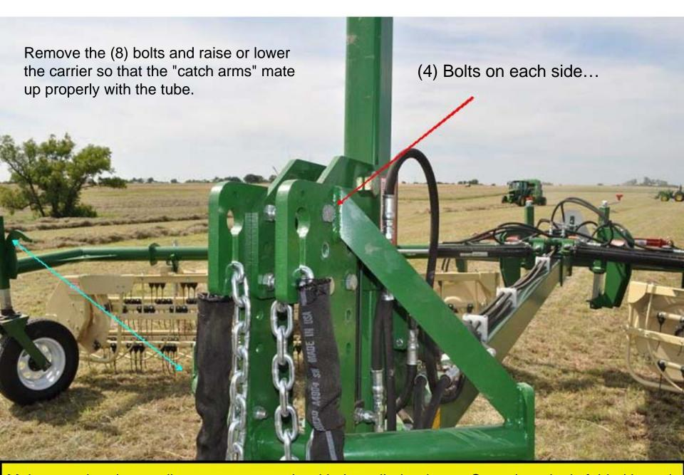
Make sure that these adjustments are made with the cylinder down. Once the rake is folded in and raised, you'll want all of the lift travel possible for transport position.
