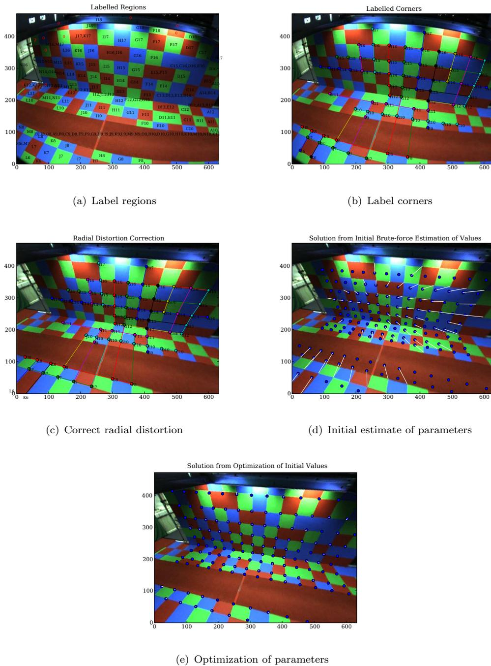
FIGURE 5.8: The steps taken to calibrate a camera
