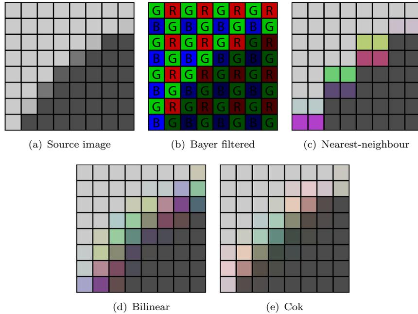
FIGURE 5.2: Filtering of image by Bayer array and recovery of colour information by interpolation
