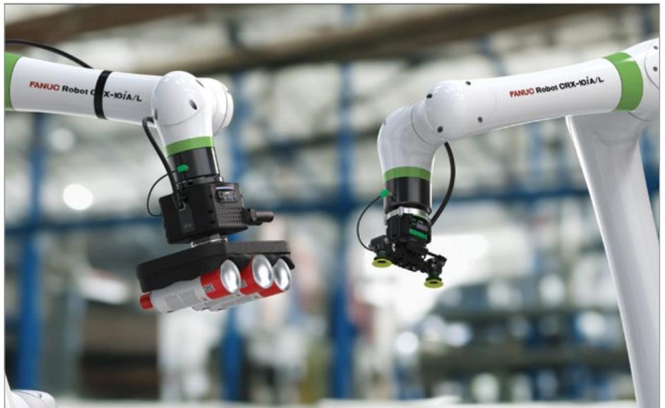
New piCOBOT® plug & play configuration for FANUC CRX cobots.
