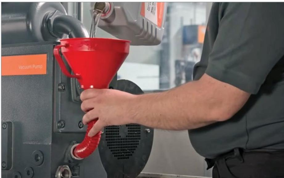
*Certain vacuum pump oils are available with improved corrosion resistance that can help you to protect your vacuum pump during wintertime.*
