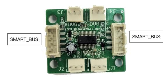
RC\_Servo board can control up to 4 RC servo. The default SMART\_IDs for these RC port are 8,9,10,11. The initial SMART\_ID (id =8) can be configured in program.
