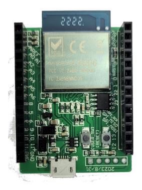
SMART\_IO\_V2 provides 12 digital I/O + 4 Analog input ports for external sensors or output in 3.3 V
