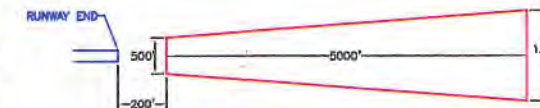
TYPICAL RUNWAY 10-28 EXISTING PART 77 APPROACH SURFACE - FULL PLAN VIEW Not to Scale
