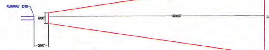
TYPICAL RUNWAY 10 PROPOSED PART 77 APPROACH SURFACE - FULL PLAN VIEW Not to Scale
