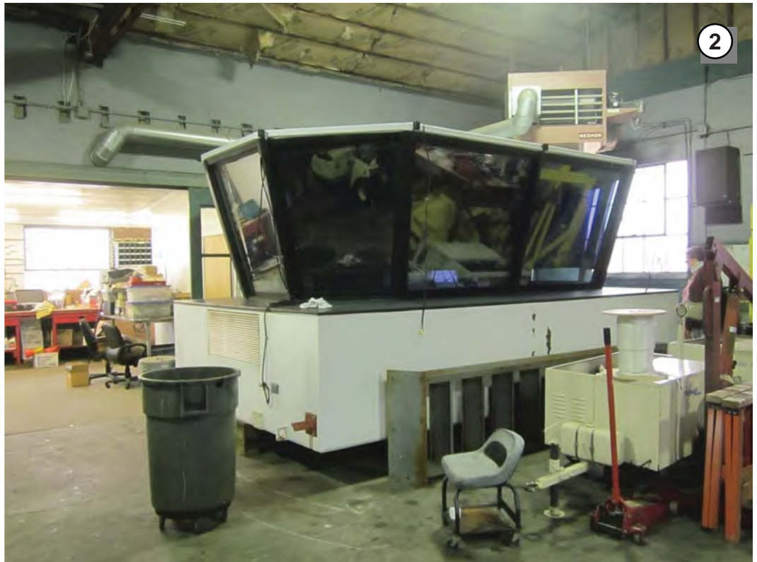
The mobile ATCT cab which, during the off-season is housed in a garage on-Airport (Field Photograph 2013-02-27 002, February 27, 2013).
