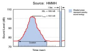
The compression of energy into one second means that a given noise event's SEL will almost always will be a higher value than its Lmax, as shown on the figure. For most aircraft flyovers, SEL is roughly five to 12 dB higher than Lmax. Adjustment for duration means that relatively slow and quiet helicopter or propeller aircraft can have the same or higher SEL than faster, louder jets, which produce shorter-duration events.
