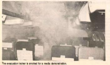
emergency equipment. This Cabin Trainer was located on an elevated level of the building, which allowed flight attendants to perform actual slide evacuations. The trainer was built upon a massive hydraulic platform, which allowed the trainer to actually move to replicate turbulence. Smoke machines also were also used to fill the cabin with smoke.
