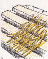
At the same time as the roof was being laid, the walls were built up further, over the roof beams, to make a parapet. This was a legal requirement, because the roof of a house was part of the used space - and people would often be up there.
