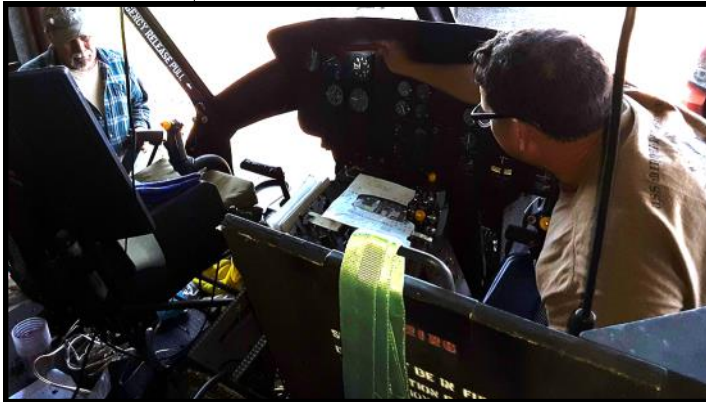
Mitch Madison (left) and Brandon Montanye (right) complete the installation of a new instrument panel in the VR Huey mission simulator. The simulator will let visitors experience a range of realistic missions and also try their hand at flying. (Helicopter Conservancy)
