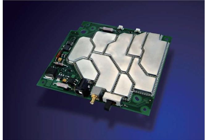
be incorporated into the shield which will improve overall device design, reduce tooling requirements, simplify post processing, and enable easier assembly. Some of these feature examples could be inclusion of strategic holes atop the shield into which potting compound is injected, making the shield a "leave in place" mold; or formed channels, which accept wires/cables to manage routing at final device assembly.
