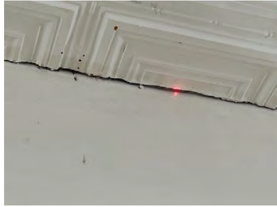
Example of air leak.
