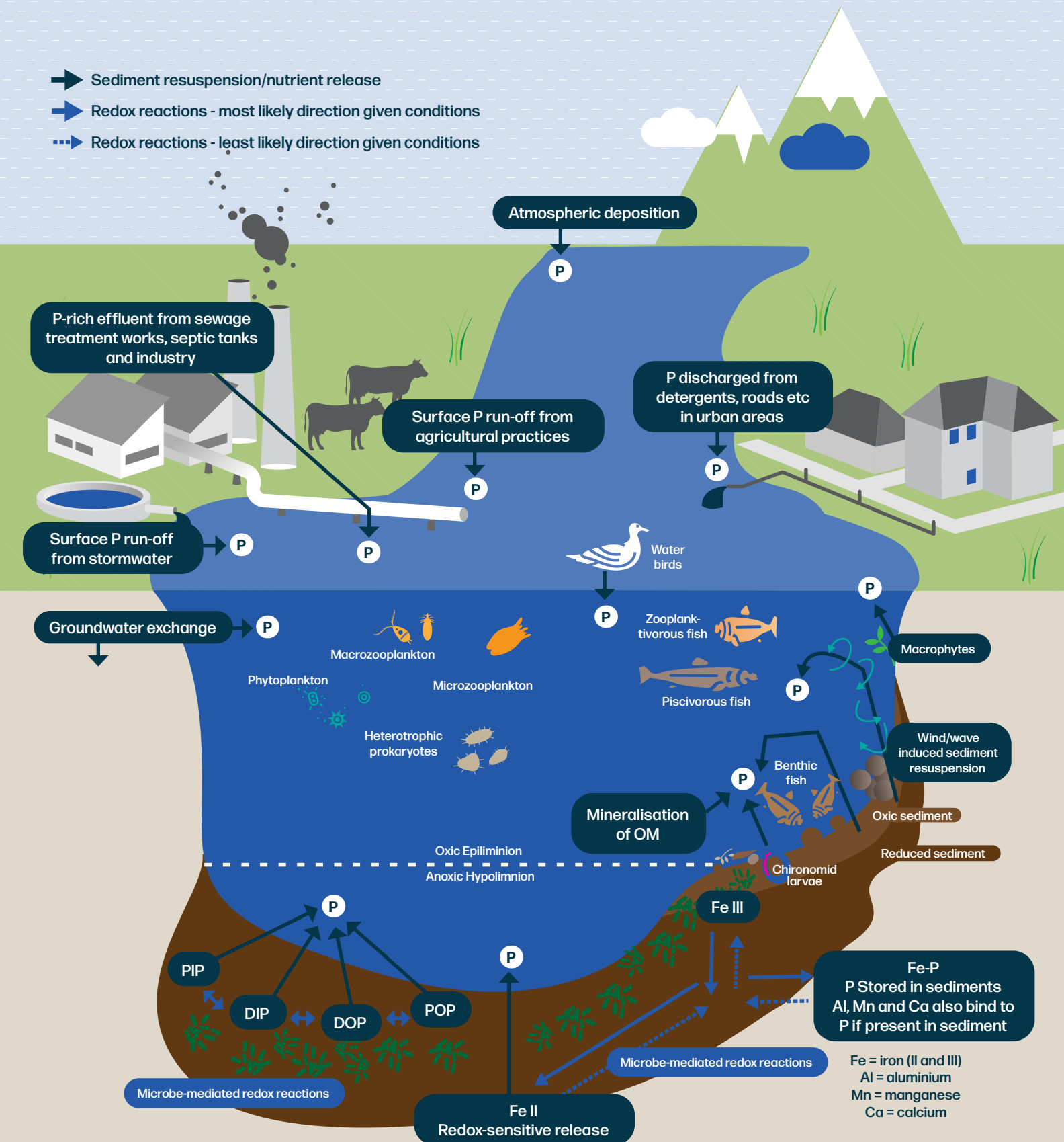
Figure 3. The main sources of phosphorus (P) to a eutrophic lake, with a focus on both external P sources and internal P load release mechanisms from chemical (redox related reactions during anoxic conditions), biological (bio-turbation - e.g. Chironomidae larvae) and physical (wind/wave action) release processes. The loss of P from a lake system include outflows, through groundwater exchange and sedimentation. P is tied in biomass in the lake (bacteria, phytoplankton, zooplankton, macrophytes, macro-invertebrates (not shown), fish and water birds) and passed through the keychain through predation/bacterivory or released back into the system through biomass degradation and excretion as organic matter (OM). The mineralisation of OM releases dissolved organic P (DOP), dissolved inorganic P (DIP) and particulate organic P (POP).
