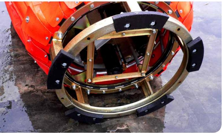
Torrentula Valve technology is capable of pilot-operated, unlimited multiple dumps, variable flow and split drops. Instant open and close valve actuation on a low power draw is achieved while retaining the superior durability and functionality of the original Bambi Bucket.
