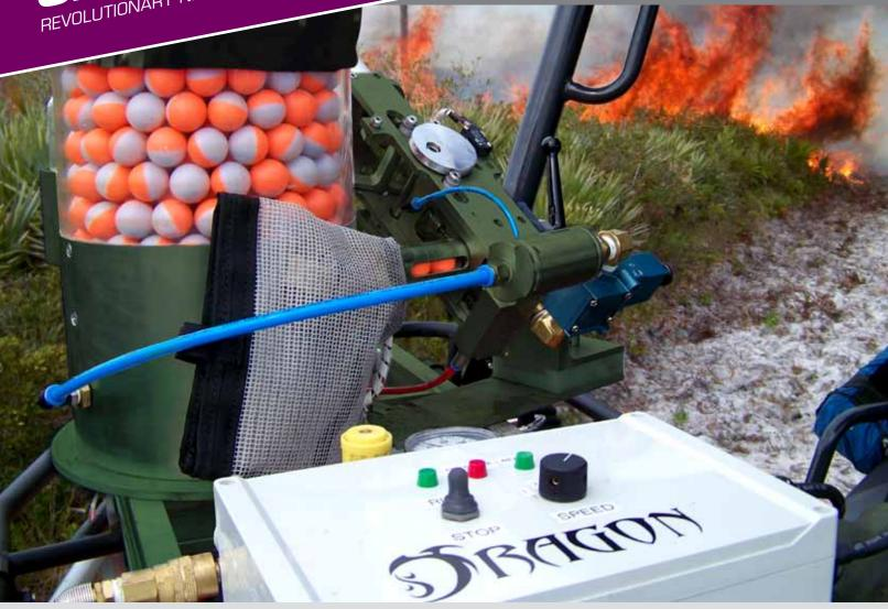
The Green Dragon® is an automated ground launcher designed and engineered for use in wildfire and land management applications such as back burns or prescribed burning. Its design represents a brand new concept for ground ignition applications using CO<sub>2</sub> or compressed air as a propellant and a simple electrically-driven reciprocating feed and firing system. The Green Dragon can be successfully mounted on several ground-based platforms including trucks, boats, ATVs and UTVs.
