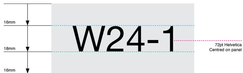
► **Fire Trail Code Sign** (uses Structure 8 / Panel H)
