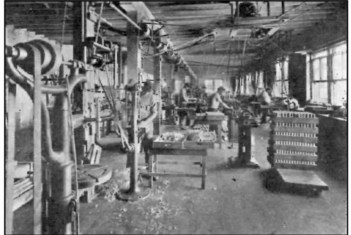
Figure 3: Typical drive shaft plus pulley structure in a factory.<sup>22</sup>
